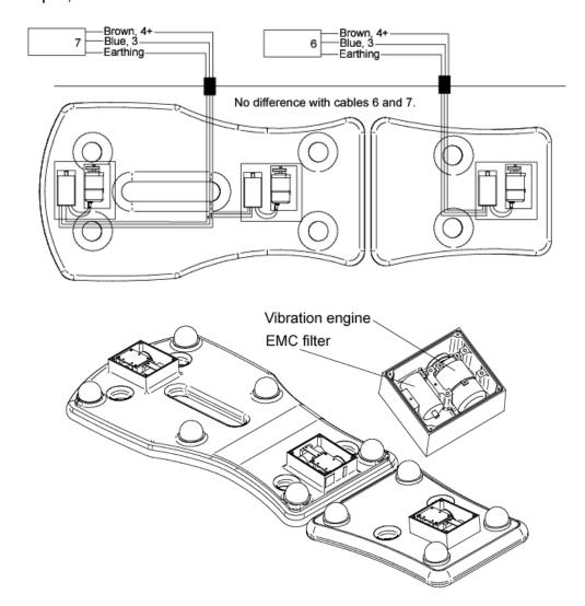
The vibration system has three (3) electrical motors with EMC filters. The motors with filters are connected to special nests on the back of the beds. Two (2) motors and filters are located on the upper bed, and one (1) motor and filter is located on the lower bed. Two (2) electrical connections for the beds are located on the capsule bottom floor.
