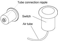
The on-off switch breaks electric input when you press it.
