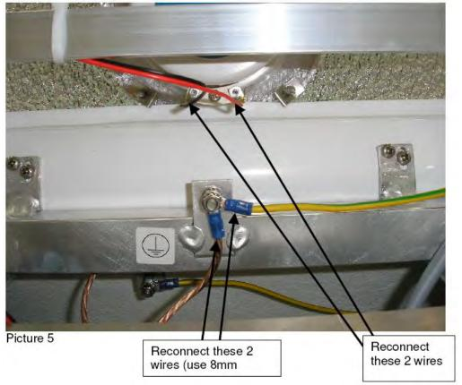
The wires that were reconnected in Steps 4 and 5 have to be attached to the aluminum frame via wire ties. Notice 5 black marks on the aluminum frame – these marks indicate the position where wire ties need to be installed to attach the wires to the aluminum frame. Snip the excess plastic off the wire tie after tightening to the aluminum frame.
