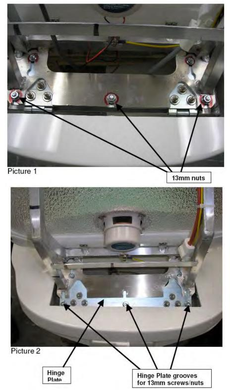
2) Position the hood so the three grooves in the hinge plate shown in Picture 2 are aligned with the three 13mm screws/nuts. Slide the hood forward so the hinge plate slides under the three 13mm nuts and the two 10mm screws are also in their groove (See Picture 3).
