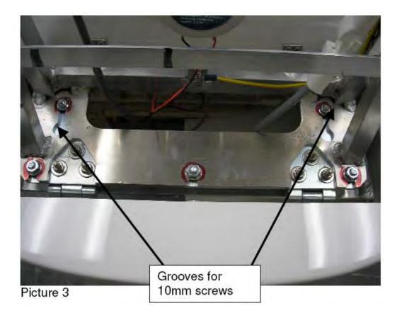
3) Ensure the hood is pushed as far forward as possible (so the screws bottom out in their grooves). Tighten the three 13mm nuts and install and tighten the two 10mm nuts.
